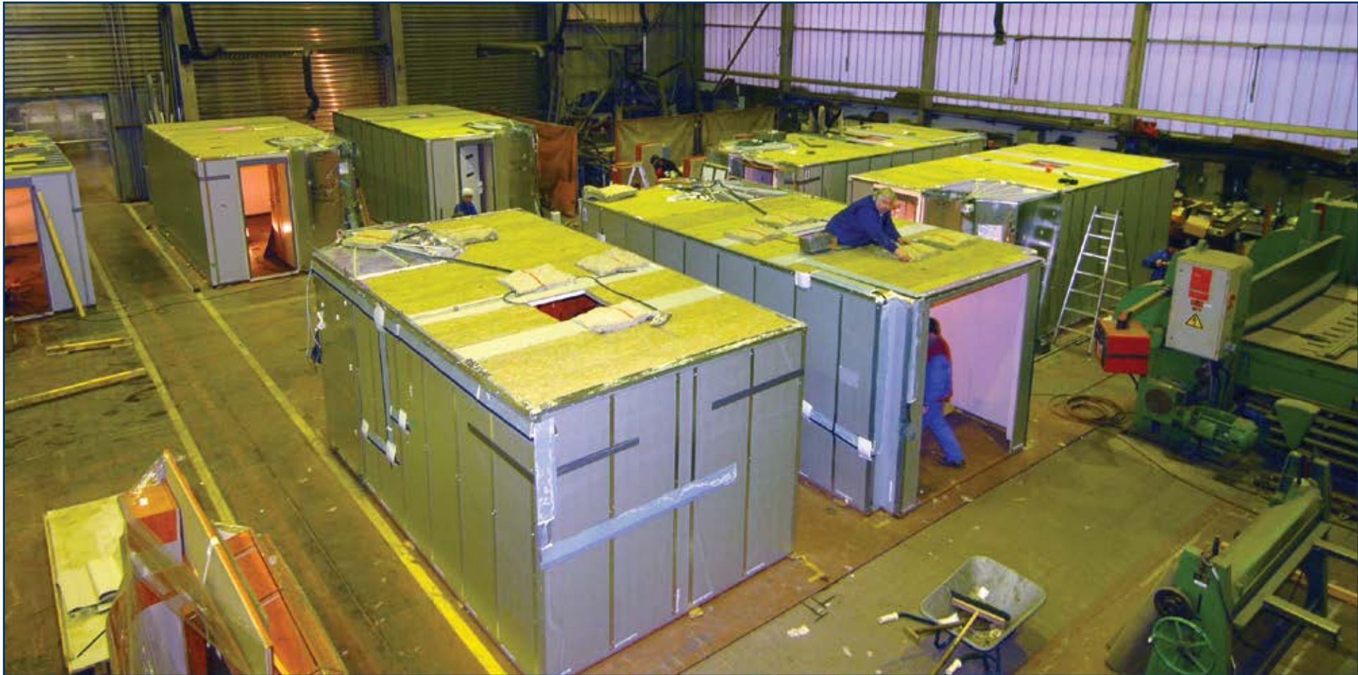
Prefabricated cabins are prepared for transport to the ship.
